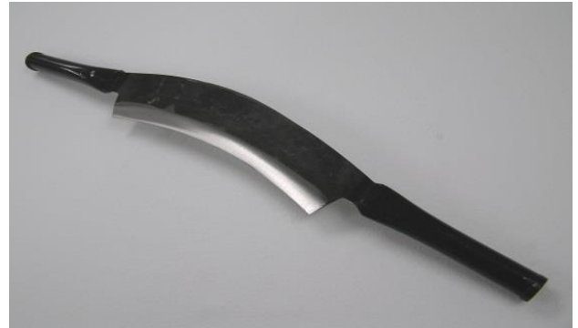
R-Type Cutter for scraping tuna skin
